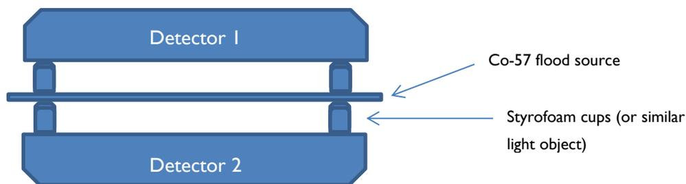
Figure 1: Set-up for extrinsic uniformity and sensitivity test, dual-head gamma camera.
