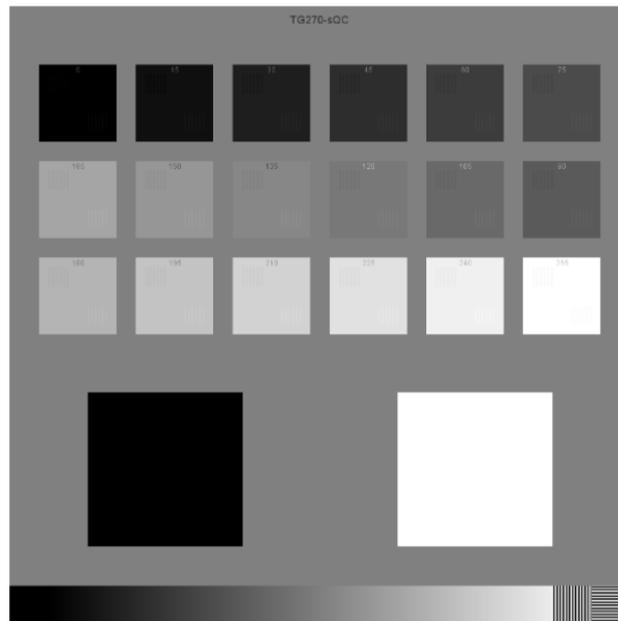
**Figure 2: TG270-sQC test pattern for quality control of CT workstation and reporting monitors.**
