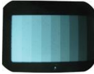
Figure 2: A reference radiograph, showing incremental increases in density. Copyright Margraf Dental.
